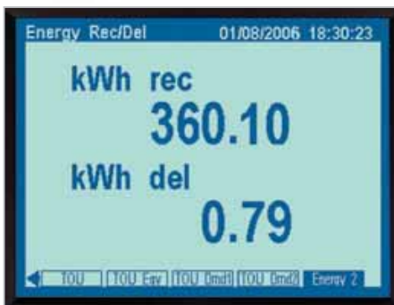
Energy received/delivered display
